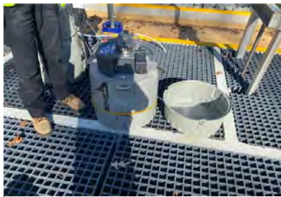
ISCO at effluent
